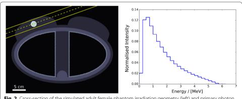
**Fig. 2** Cross-section of the simulated adult female phantom irradiation geometry (left) and primary photon energy spectra of the simulated 6 MV Varian Linac source taken from Sheikh-Bagheri and Rogers (2002) (right). The solid and dashed yellow lines represent the outer edges and central axis, respectively, of the 30-mm-diameter circular non-diverging photon beam rotated 20° off-axis focused at the two-compartment tumour centre located in the left breast
